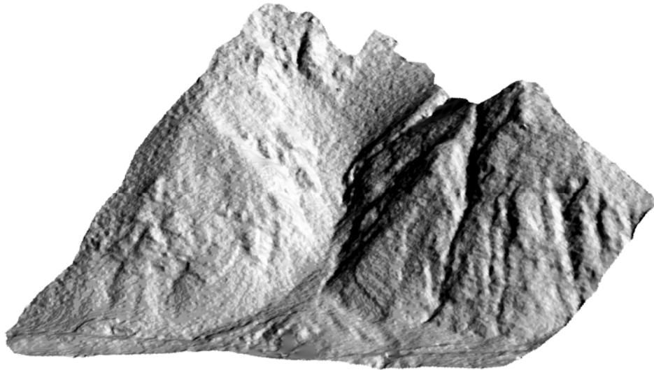
Fig. 6: DEM (resolution 2m) derived from stereo images for the study area Guido A, after removing peaks and holes. The international road is well recognizable at the lower edge of the DEM. Its length represented in the dataset is about 800 m, the elevation difference 700 m.
